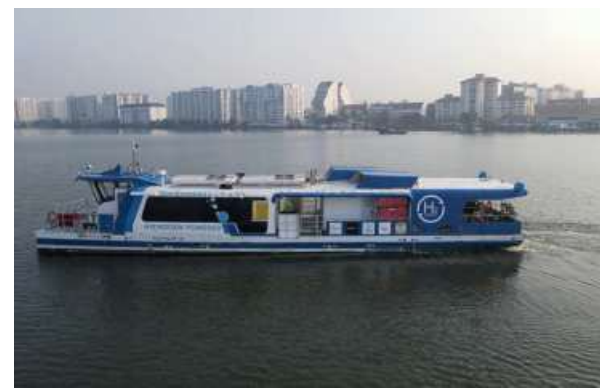
Brand new: Built by the Cochin Shipyard, the hydrogen fuel cell ferry boat can carry up to 50 passengers. SPECIAL ARRANGEMENT
