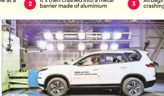
The most common crash test is the offset frontal impact (above)
