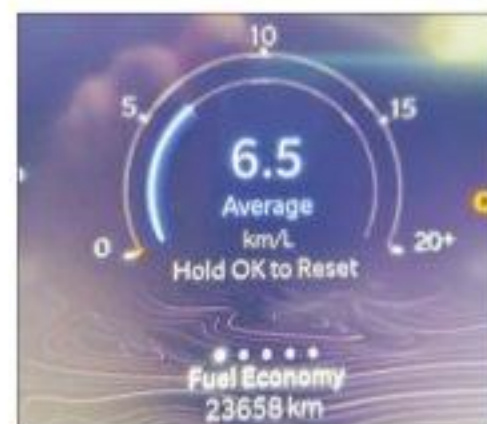
Fuel efficiency is poor — it was about 10 km/litre on highways, and 6.5 km/litre in the city
