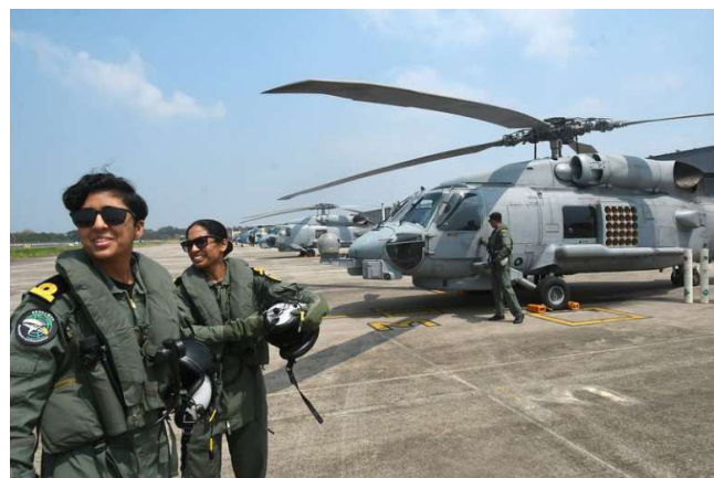
Latest addition: The Navy's newly inducted MH 60R Seahawk multi-role helicopters seen at INS Garuda in Kochi on Thursday. The Navy is set to commission MH 60R, which is capable of firing torpedoes, missiles and Advanced Precision Kill Weapon System rockets. The self-protection suite on the helicopter comprises chaff and infrared flares, which can be deployed automatically upon detection of threat. TULASI KAKKAT
